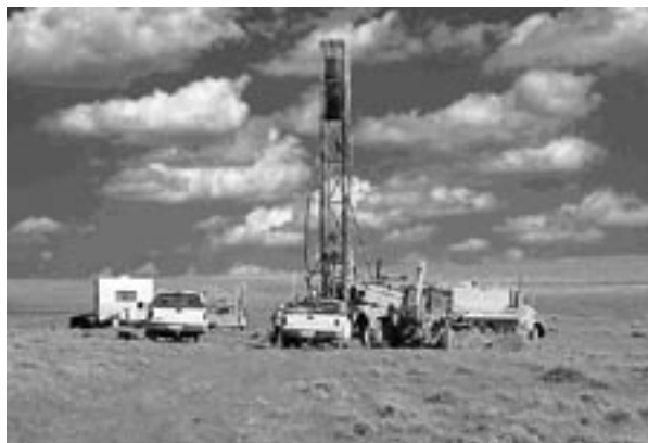
Truck-mounted drill rig used by gas developers for shallow drilling of coal-beds in the Powder River Basin.
