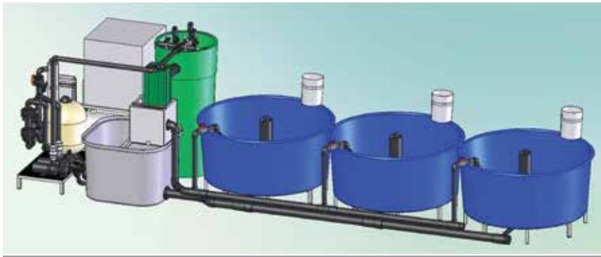
Recirculating aquaculture systems used as drought safe haven by the California Department of Fish and Wildlife.
