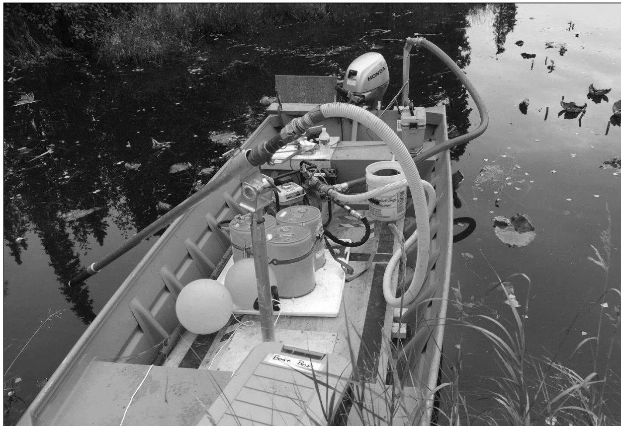
Figure 5.—Outboard-powered skiff with spray turret.
