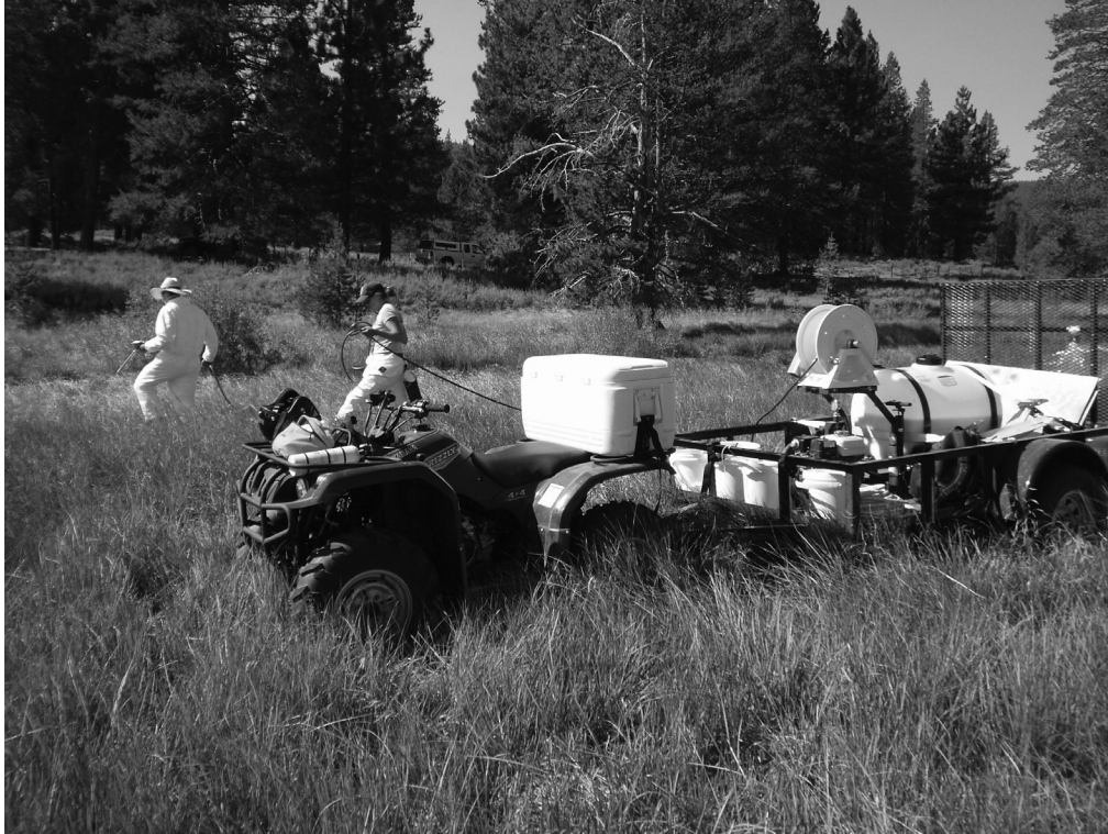
FIGURE SOP 12.5. High-pressure sprayer is transported to site with an ATV. Spray is delivered to the site using a high-pressure hose mounted on a hose reel. Note that person carrying the hose is not wearing a particulate respirator since she is not currently spraying (Photo credit: Bill Somer, California Department of Fish and Game).
