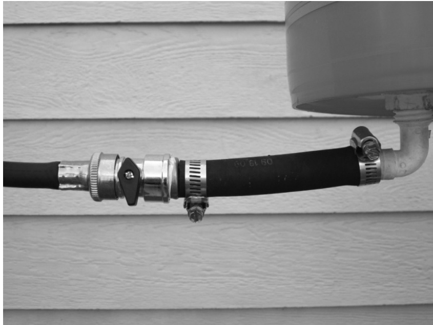
APPENDIX FIGURE 3. Drip bucket reservoir showing hull fitting, 1/2 inch hose with clamps, cut-off valve, and garden hose attachment.
