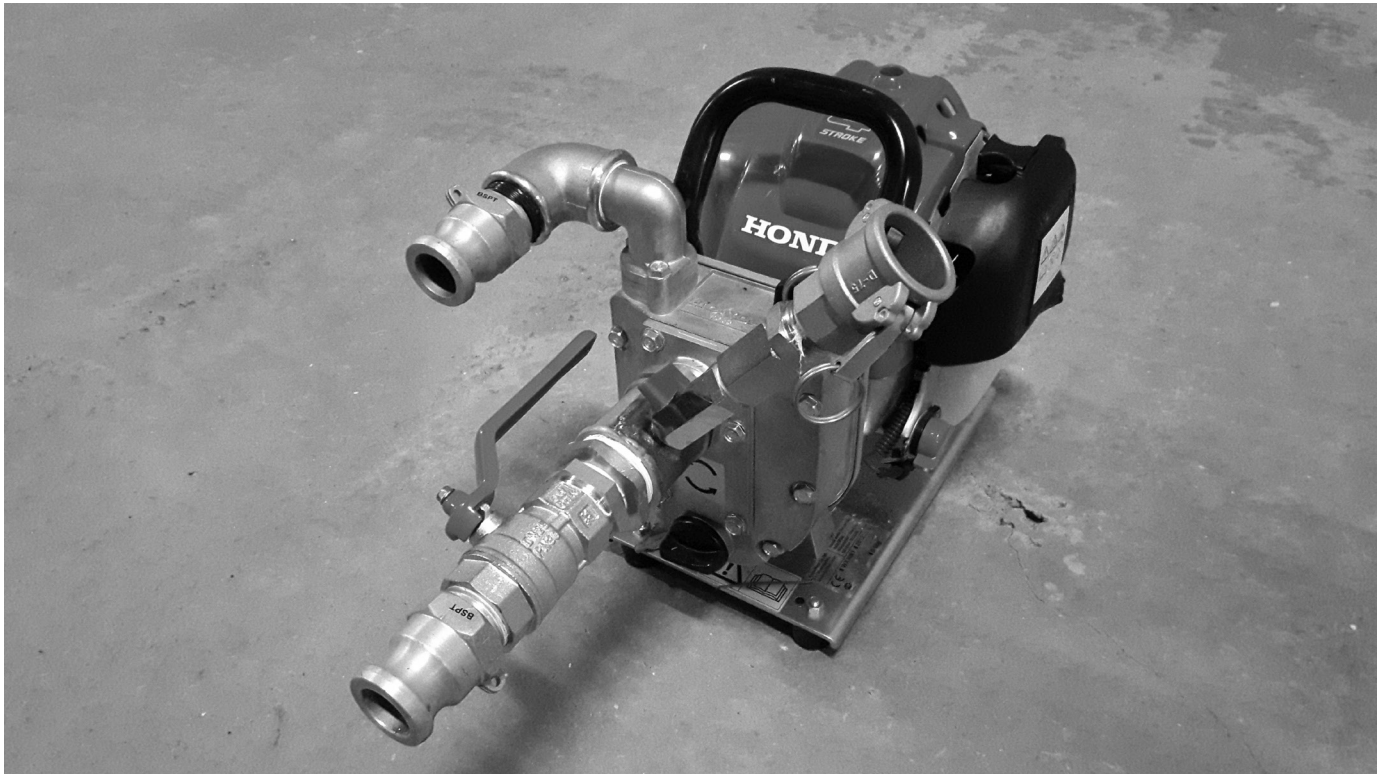
FIGURE SOP 13.1. Small portable water pump used for the application of Vectocarb/CFT Legumine slurry.
