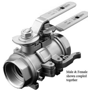
FIGURE SOP 8.3. An example of a dry disconnect valve showing the two halves coupled together with cam arms. Two interlocking handles make opening and closing easy. When liquid is flowing, disconnect valve halves cannot be uncoupled without turning handles to closed position. When disconnect valve halves are apart, handles cannot be turned to open position.
