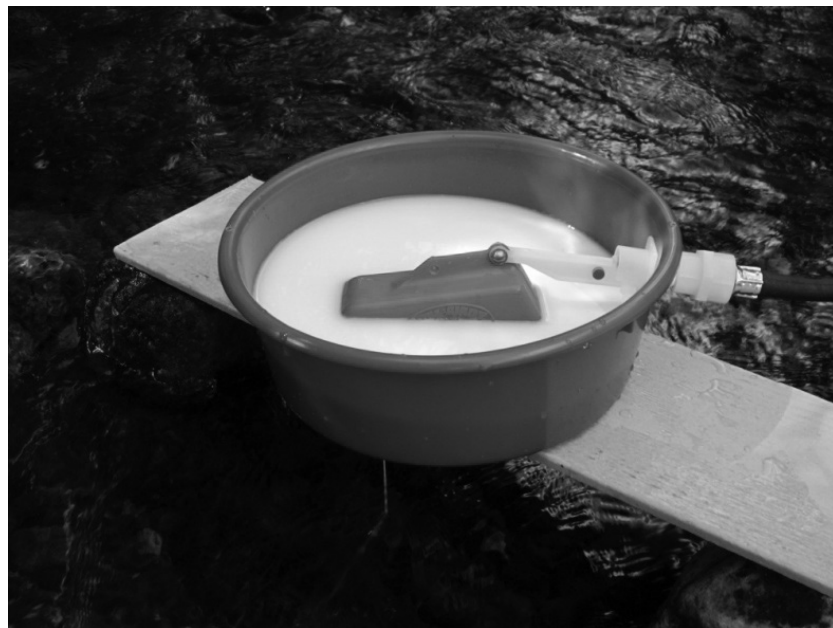
APPENDIX FIGURE 4. Dog watering bowl reservoir and float in operation. Feeder garden hose from drip bucket reservoir on right side of photo.
