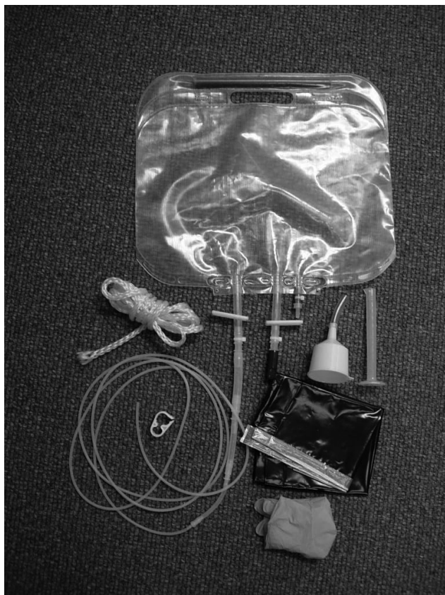
APPENDIX FIGURE 7. Photograph of plastic reservoir (Labtainer BioProcess Container) with Tygon tubing attached and accessories, including funnel, black plastic bag, nitrile gloves, 10 ml volumetric cylinder, and rope for hanging bag.
