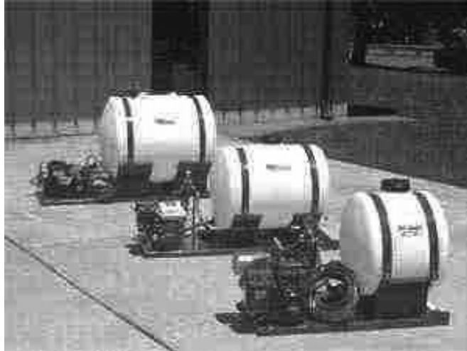
FIGURE SOP 12.3. Typical gasoline-powered high-pressure sprayer units. Note all service containers must have labels that identify the following: (1) name and address of the person or firm responsible for the container, (2) the identity of the pesticide in the container, and (3) the pesticide signal word (i.e., “DANGER”, “WARNING”; per SOP 4.1).
