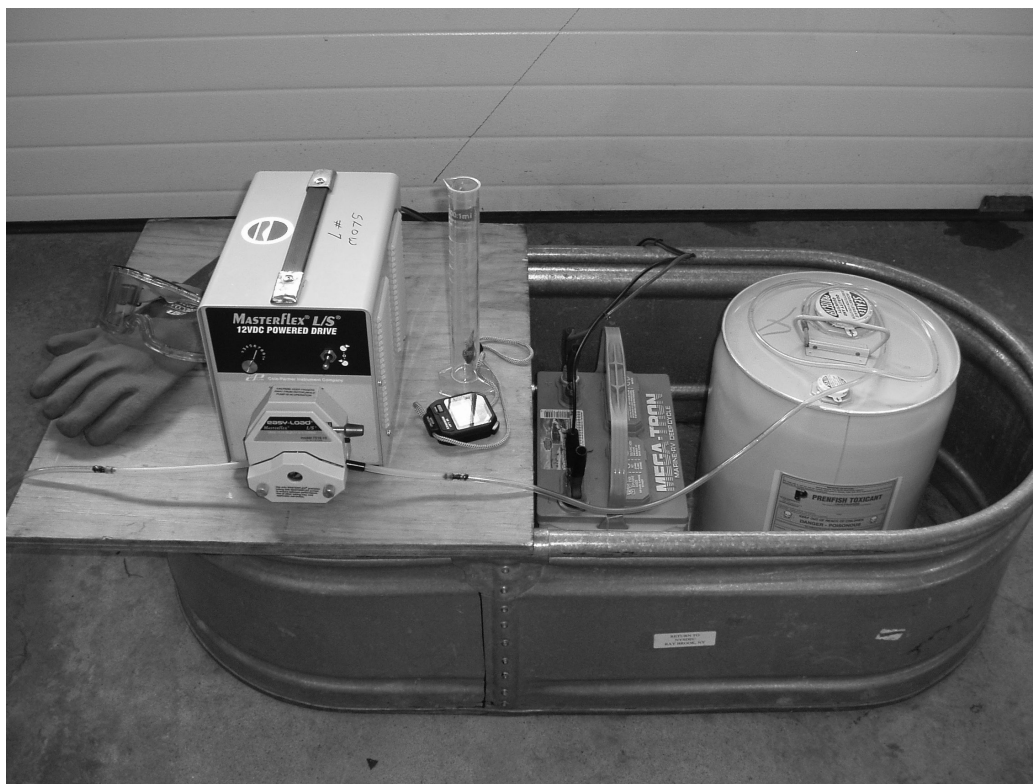
FIGURE SOP 11.2. Masterflex peristaltic pump set up in secondary containment, personal protective equipment on hand, stop watch and graduated cylinder.
