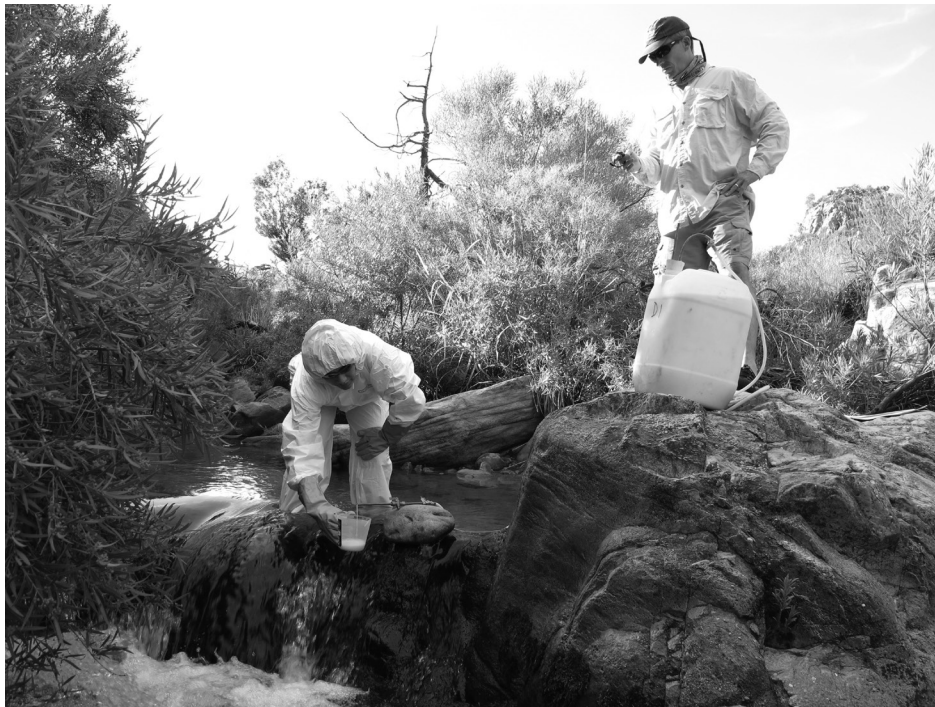
FIGURE SOP 11.1. Checking the emission rate from a drip can using a measuring cup and a stop watch.
