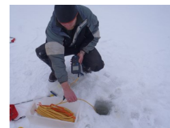
Winter dissolved oxygen testing - International Falls Area Fisheries Office
