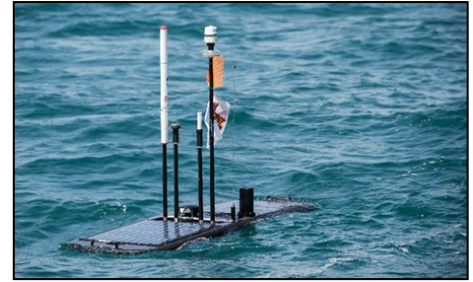
R/V Blackbeard, an SV2 wave glider outfitted with an Innovasea VR2C acoustic receiver on a mission tracking Southern Flounder offshore of North Carolina.
