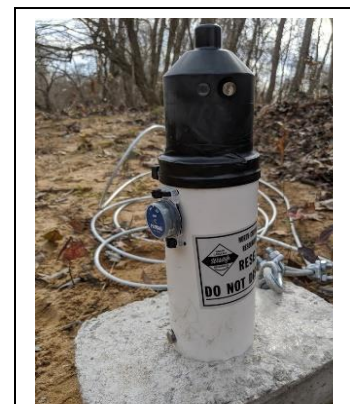
Passive acoustic receiver.
