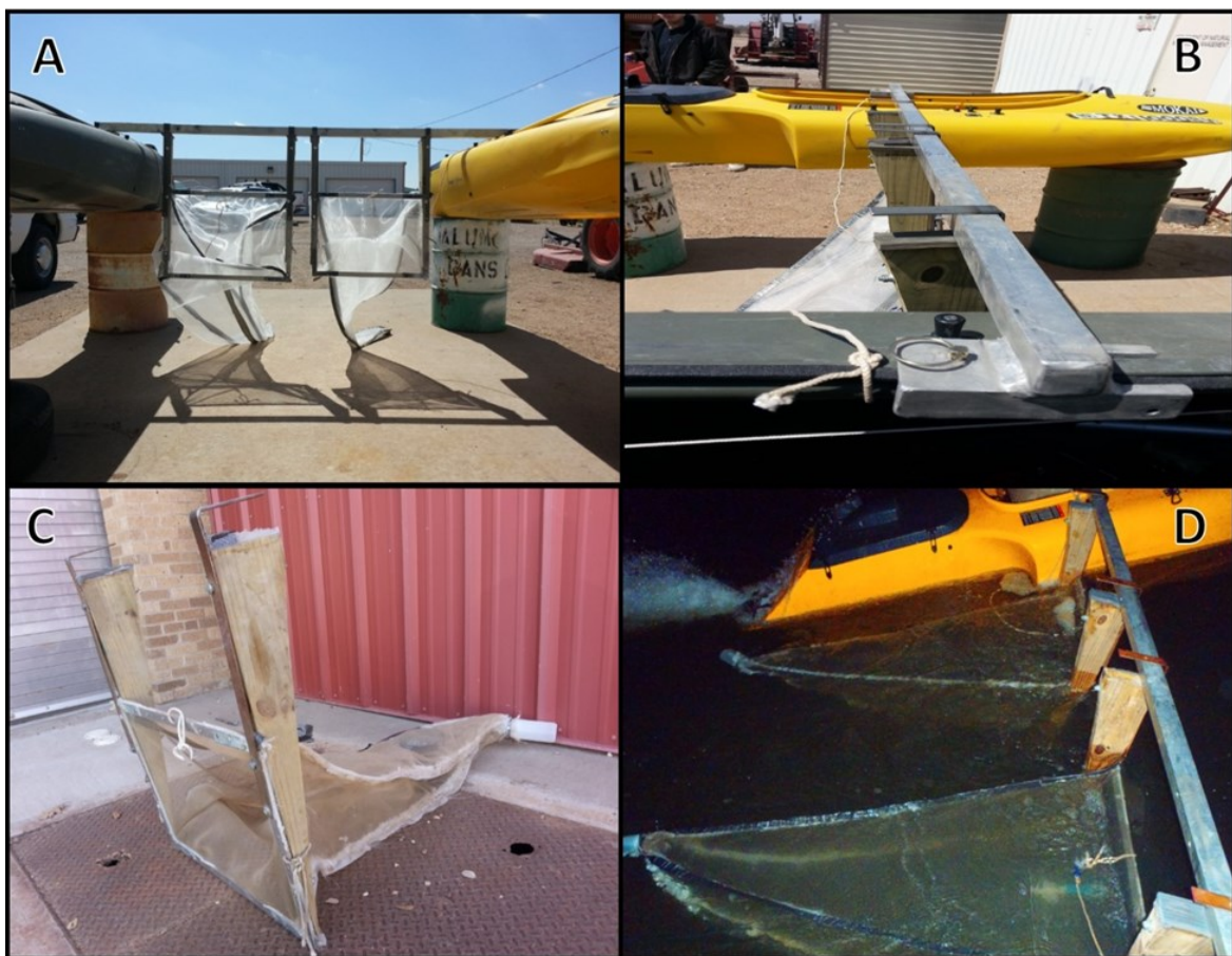
Figure 3. Paired pushnet setup and design used in the Trinity River, Texas to collect larval fish in the main channel and backwater habitats. A) Two jet-propelled kayakers connected with an aluminum bar and two modified pushnets hung from the center. B) Pushnet harness was designed so when in operation the wooden wedge would pinch against the aluminum bar and maintain their position in the water column. A metal pin (pictured) was used to keep the aluminum bar from sliding back during operation and a clamp (not pictured) was used to keep the bar from rotating on the gunwale. Additionally, a rope was connected to the gunwale and the top frame of the pushnet to reduce the chances of losing a net when debris was encountered. C) Modified pushnet built from 500- \mu m netting and silicone to seal the seams. D) Paired pushnets deployed during a transect with flowmeters attached at the mouth of each net.
