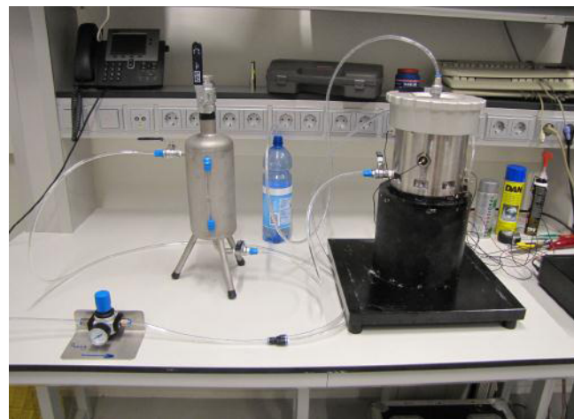
Fig. 1. The device which was developed to expose fish larvae to loud impulse sounds.
