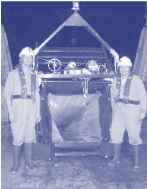
David Holliday and Lynnath Beckley with the multiple opening and closing EZ net they used off the RV Southern Surveyor to examine vertical distribution of fish larvae in the Leeuwin Current eddy field.
