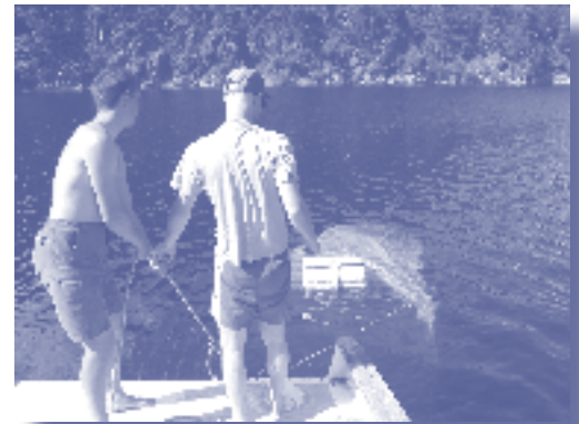
Photo.3. Sampling of perch larvae and juveniles using ichthyoplankton trawl (mouth opening 2 x 2 m, mesh- size 1 x 1.35 mm).
